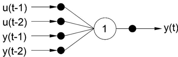
Figure 8. Nonlinear ARX model structure of the wear process
