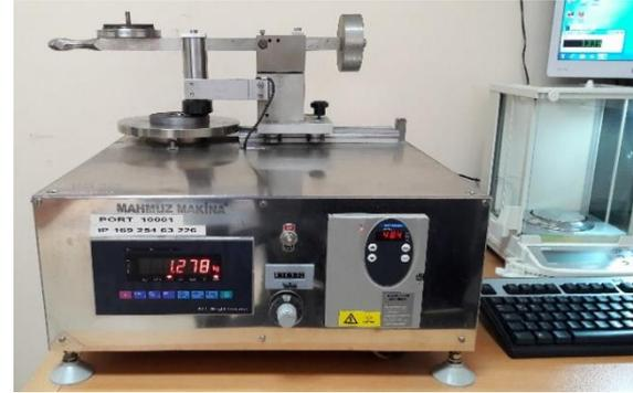
**Figure 6.** Pin on disc test apparatus
