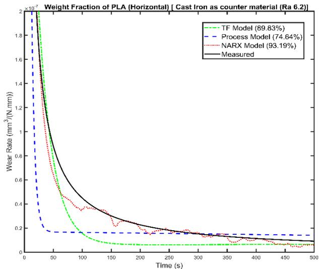
**Figure 17.** Weight fraction against cast iron (horizontal orientation)
