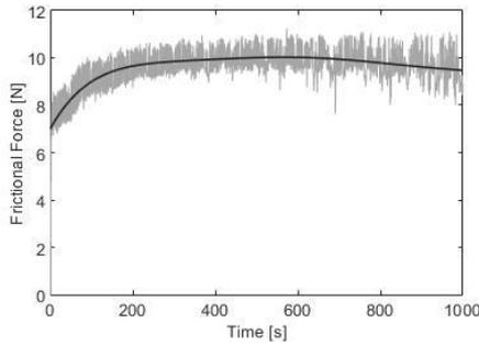
**Figure 12.** Horizontal Orientation- Cast iron as counter material (Ra 6.2)
