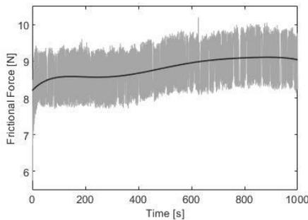
**Figure 14.** Horizontal Orientation- Steel as counter material (Ra 3.2)
